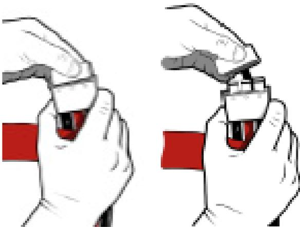
The air hoses are connected simply by hand. No special tools required.
