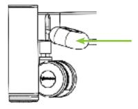
The bed bottom frame is equipped with four casters. Empty the head of the bed and make sure that the casters at the head & rear of the bed are active.
